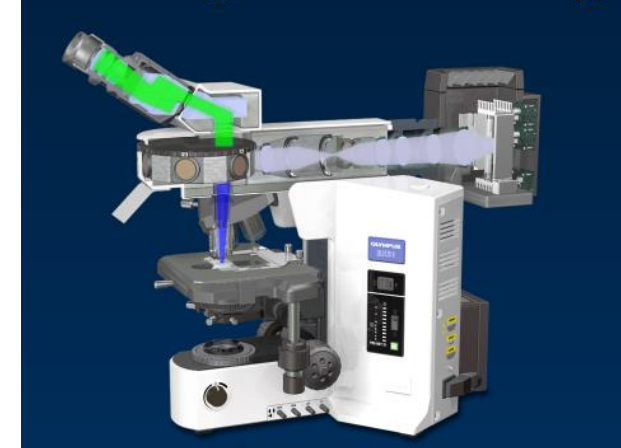
Reflected Light Fluorescence Microscopy
