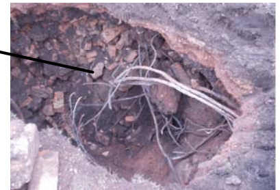
Debris (high resistivity) with metal waste (low resistivity)
